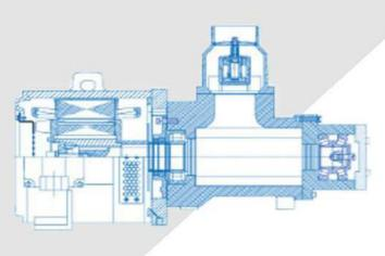
Oil-cooling pendulous coaxial structure with no bearings (ZLS10i - ZLS100i)
